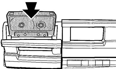
Insert a tape with the exposed side down. Push the cassette holder to close.
